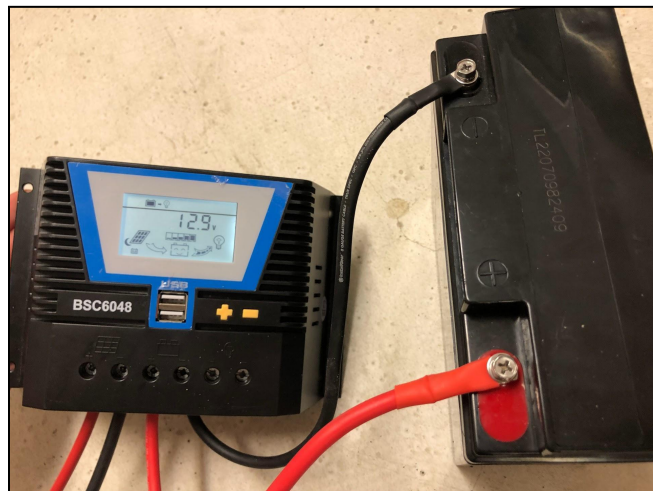
Unscrew the terminal screw on the battery
