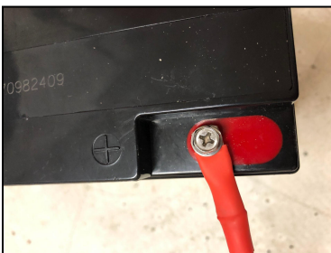
Put the screw through the O-ring and tighten
