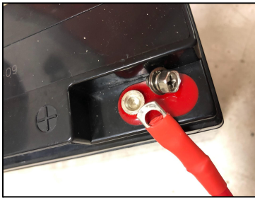
Unscrew the terminal screw on the battery
